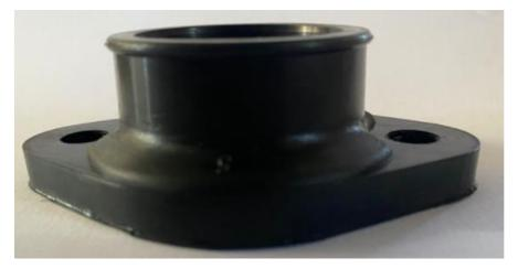
i. Exhaust Manifold: The only exhaust manifold permitted is as per photos and dimensions below. No material may be added or removed. The Exhaust Manifold gasket as supplied must be fitted at all times.
